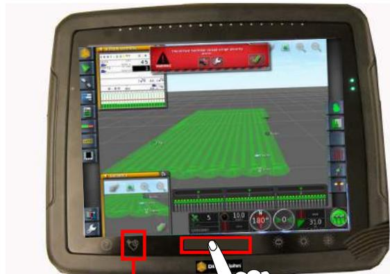
Press Eject USB button before removing USB memory device
