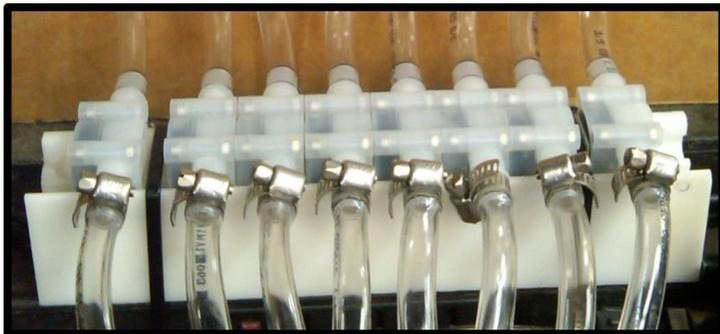
This is an example of an 8 Row System Using Hose Barb style flowmeters
