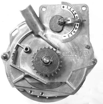
The second part of the metering box is called the **cover**. The cover is secured to the main housing by 2 wing nuts. The components on the outside of the cover are a control window and trap door. The components on the inside of the cover are a metal shutter, and ejector block.
