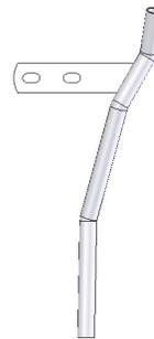
7085.GA Mounts on the left hand side of the unit, with the same bolts that attach the disc scraper. It deposits material down in the seed trench behind the seed tube. The top of the tube points straight up.
