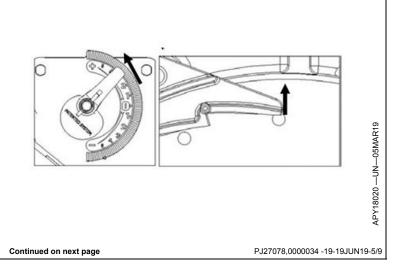
Setting for SMALLER SEED the hole on meter-box opens which reduces suction and the SCRAPER moves towards the seed disc hole.
