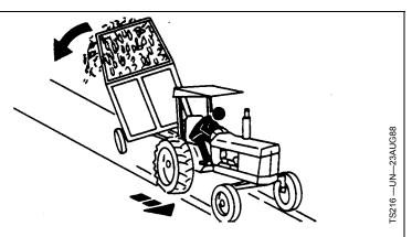
tractor must be heavy and powerful enough with adequate braking power for the towed load. Use additional caution when towing loads under adverse surface conditions, when turning, and on inclines.
