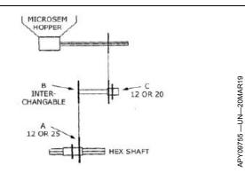
A—Double sprocket on hex shaft - driven 1 C—12 or 20 tooth sprocket
