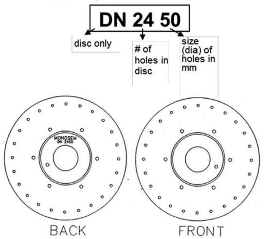
The size of the seed disc is engraved on the back of the seed disc. When ordering seed discs, the prefix DN indicated the disc only. The prefix DC indicates the complete disc with brass agitator (6212.a). The first two numbers of a four number series indicates the number of holes in the seed disc. The second two numbers indicates the size (diameter) of the holes.
