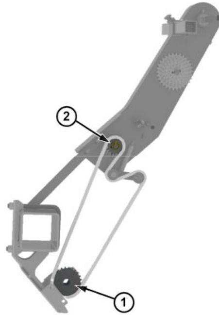
sprocket (1) and the interchangeable sprockets (2). The chart provided will assist with the setting and indicates the sprockets to be used for the principle commercial products. The provided information is a recommendation only.
