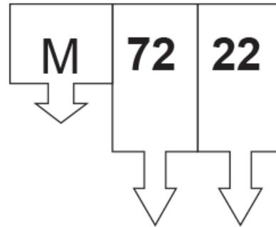
Example, Seed disc M 7222 has 72 holes, each hole having a diameter of 2.2 mm.
