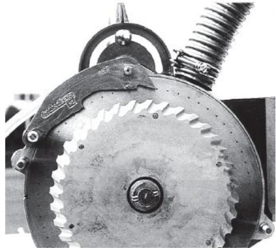
The lever raises or lowers the scraper over the seed disc holes.
