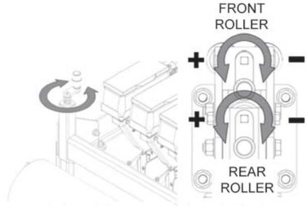
*Depth adjustment knob and Linkage adjustment knobs*
