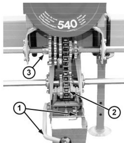
To change the seed spacing, push the idler lever, lock its pawl (1) then align to the proper sprocket combination (2). The small upper sprocket cluster is fitted with a set bolt (3), which should be tightened to avoid any sliding of the cluster.
