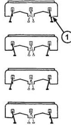
**The primary adjustment** is set by using the lower double sprocket. **The final adjustment** is made by using one of the sprockets of the upper sprocket cluster. Outputs can thus be obtained between approximately 80 to 350 lbs/acre (80-350 kg/ha).
