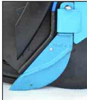
v-slice insert with starter tube
