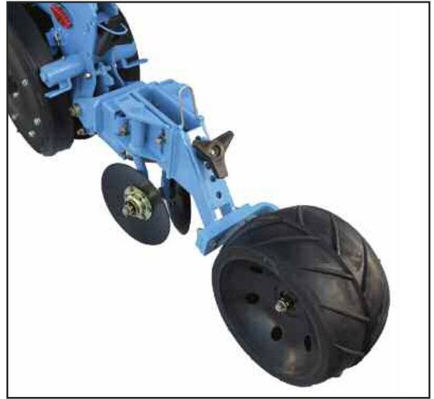
Flat Press Wheel with disc closing system
