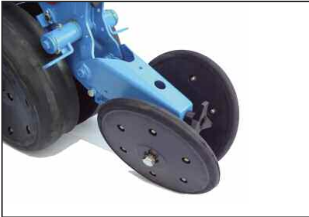
V-Press Wheel screw adjust / rubber closing wheels
