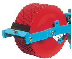
Cage rear wheel waffle marks bed top to promote soil cracking for seed emergence in crust conditions.
