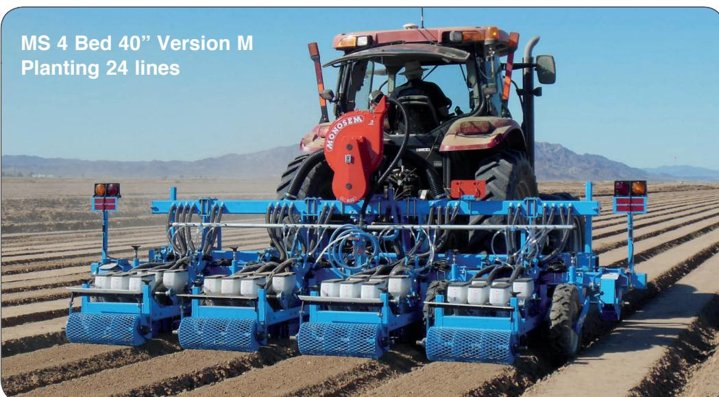
The Version M is a multiple meter row configuration designed for very close seed lines. Seed lines as narrow as 1" apart across the bed top. Perfect for onions, carrots, spinach, and leafy greens where high populations and narrow seed line spacing is desired.
