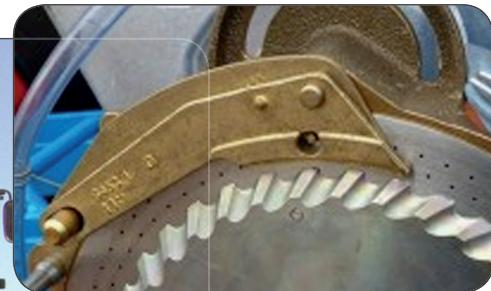
The secondary scraper is used on a Version C to singulate seed on the lower set of seed disc holes.
