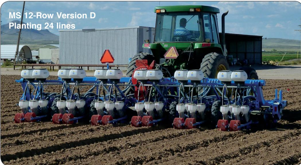
The Version D is a row unit with two staggered metering boxes on one carrier unit. Each meter has a single or optional twin seed lines to allow for multiple combinations of seed lines. Seed line spacing in the double row unit can be adjusted from 3" to 4.5".
