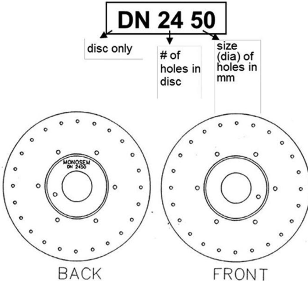
The size of the seed disc is engraved on the back of the seed disc. When ordering seed discs, the prefix DN indicates the disc only. The prefix DC indicates the complete disc with brass agitator (6212.a). The first two numbers of a four number series indicates the number of holes in the seed disc. The second two numbers indicates the size (diameter) of the holes.
