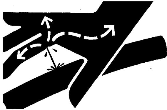
fluid openings until ready to make connection. Foreign material damages the hydraulic system.
