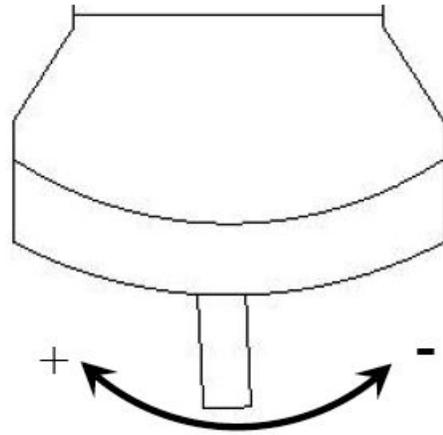
Adjust the metering gate accordingly until the desired rate is achieved. Zero for minimum output while 45 for maximum output.
