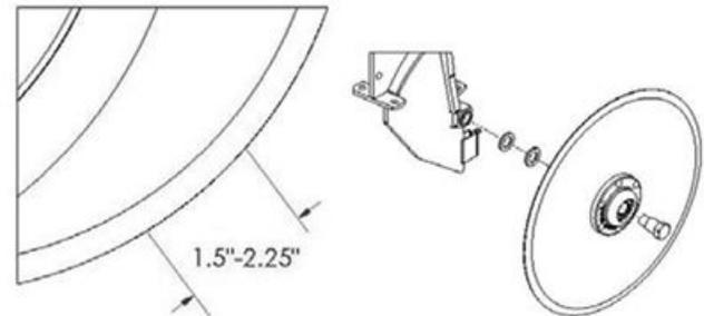
adding or removing shims to the spindle bolt. The spindle bolts should be torqued to 100 ft-lbs.
