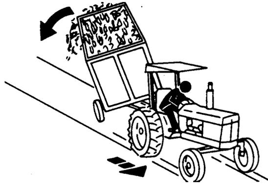
tractor must be heavy and powerful enough with adequate braking power for the towed load. Use additional caution when towing loads under adverse surface conditions, when turning, and on inclines.
